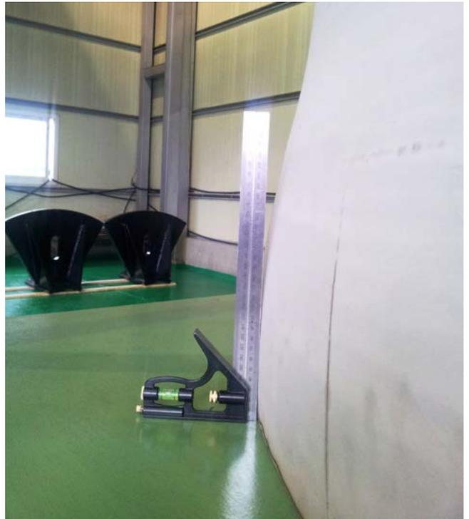
▲ Expanded Pipe View / ASTM A240 TP 321H / 20T
