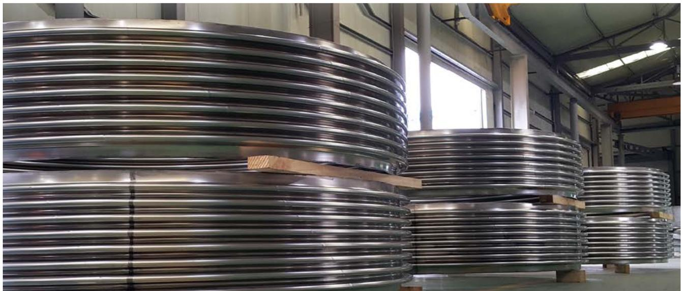
▲ Expansion joints are manufactured in a variety of austenitic stainless steels, nickel alloys and other materials such as Hastelloy and Corten. Selection of the bellows material is one of the single most important factors to consider in the design of an expansion joint.
