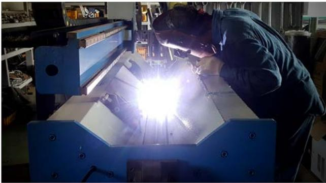
▲ Automatic Longitudinal Seam Welding Machine
