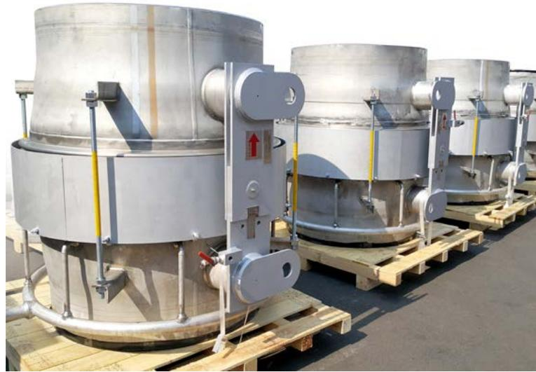
▲ Expanded Single Hinge Type Expansion Joints
