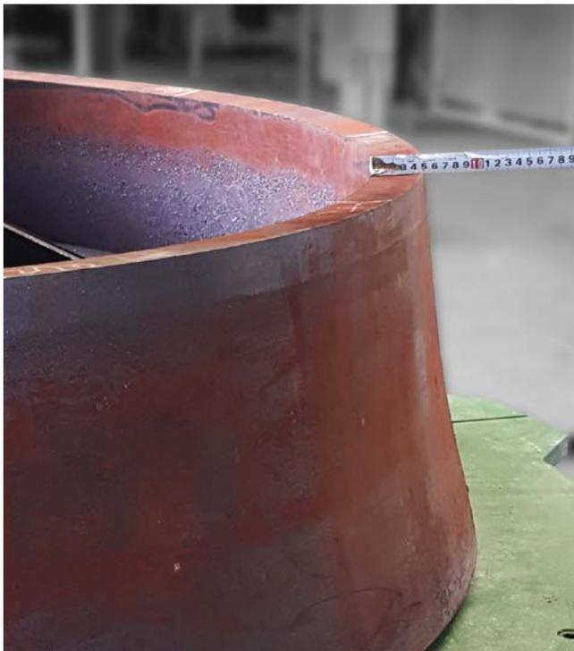
▲ Thickness Measurement (52mm) / ASTM A516 Gr70
