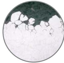
Intergranular corrosion. (200X)
